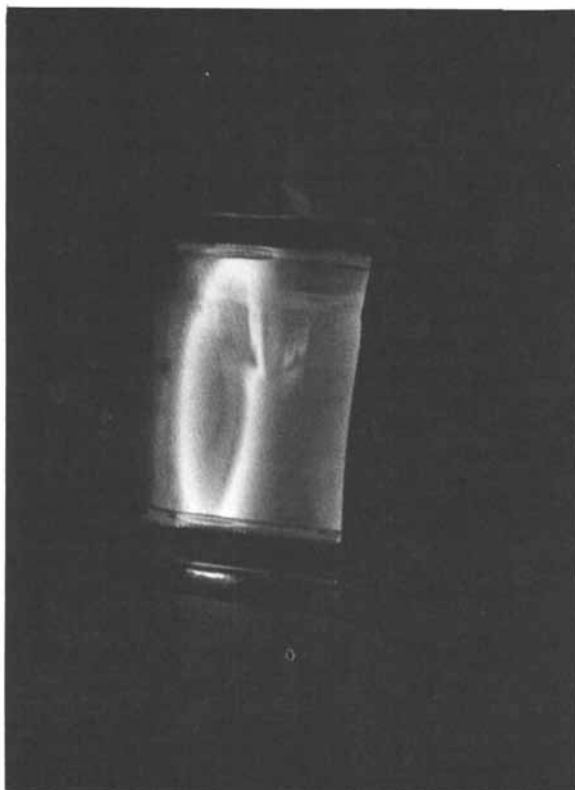
Figure 2. Photograph of an audio frequency glow discharge in the magnetic field. The pressure is 50 mtorr, current is 50 mA., N_2 gas is employed.
